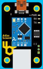
Using **BNC with Terminal Screws**, you can easily connect the Industrial ORP Probe to our **EZO™ ORP Circuit** via our **Electrically Isolated USB EZO™ Carrier Board**.
