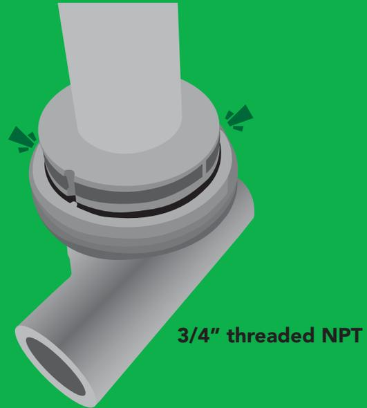
Line up the grooves and snap the probe into the pipe fitting.
