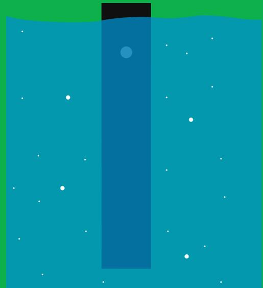
The entire conducting area must be submerged in order to get accurate readings.
