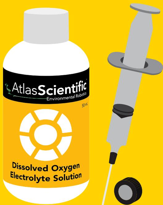
During usage, a small amount of electrolyte solution within the dissolved oxygen probe will deplete. In this case, you will need to add more solution into the probe. **To add more electrolyte solution:** carefully unscrew the probes membrane cap. Using a needle and syringe, withdraw 2mL of electrolyte solution. Insert the needle into one of the four holes surrounding the silver cathode. Inject solution until it leaks out one of the fill holes. Screw membrane cap back onto probe.
